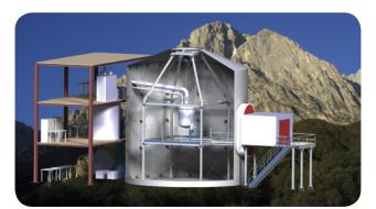
Figure 13. Rendering of the XENON1T direct detection dark matter experiment in construction at the Gran Sasso underground laboratory (LNGS) in Italy.
