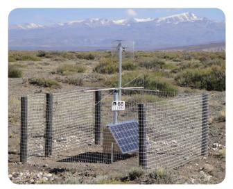
Figure 8. A detector station of AERA at the Pierre Auger Observatory to measure the radio emission from extensive air showers.
